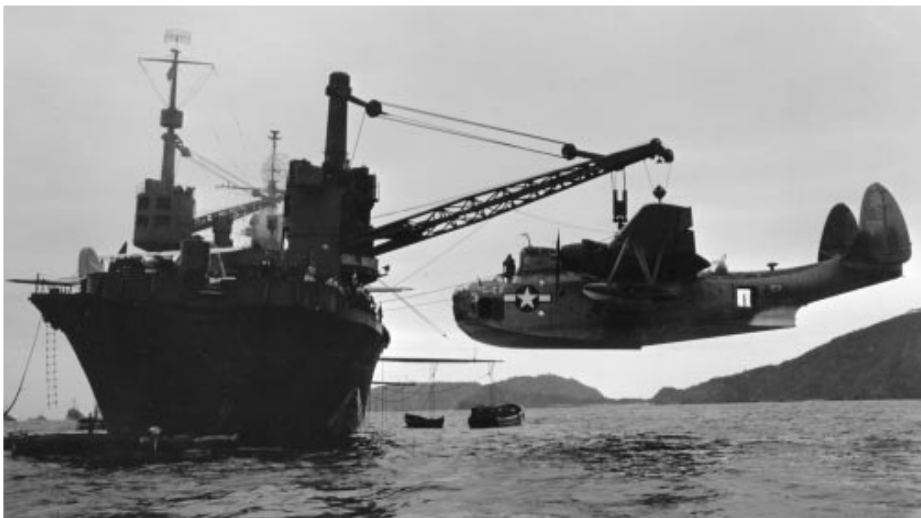
Hoisting PBM Mariner aboard tender. Normal servicing was performed from boats 428461
