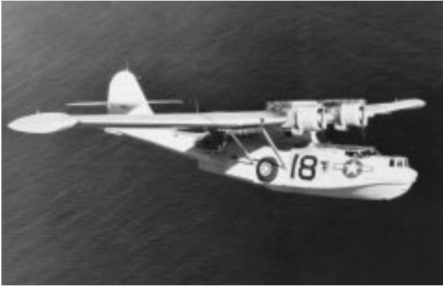
PBY-5A, amphibious version of the Catalina flying boat, carries retro-rockets for antisubmarine warfare 700504
