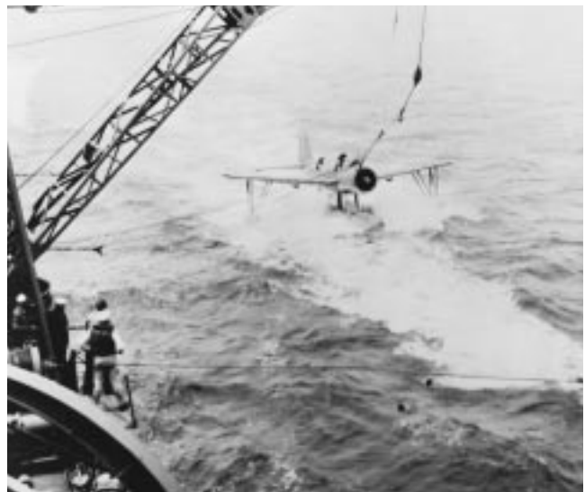
An OS2U Kingfisher is taxied onto the plane net for an underway recovery by a cruiser 299540
