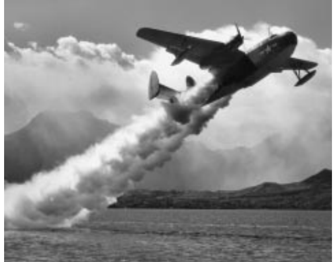
Launching a PBM Mariner, a dramatic demonstration of the utility of newly developed jet-assisted takeoff (JATO) 415346
