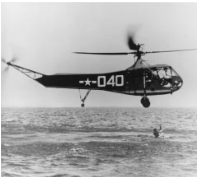
Coastguardsmen test capability of Navy's first helicopter, HNS-1, for air-sea rescue at NAS New York 1061902
