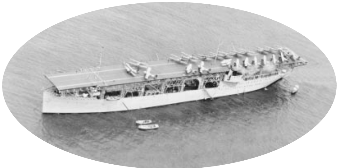
The first carrier, Langley, converted from the collier, Jupiter, with fighters and torpedo planes aboard 185915
