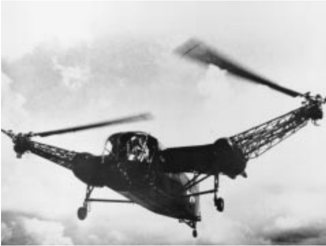
Twin rotor XHHD-1 designed for helicopter flight development 395920
