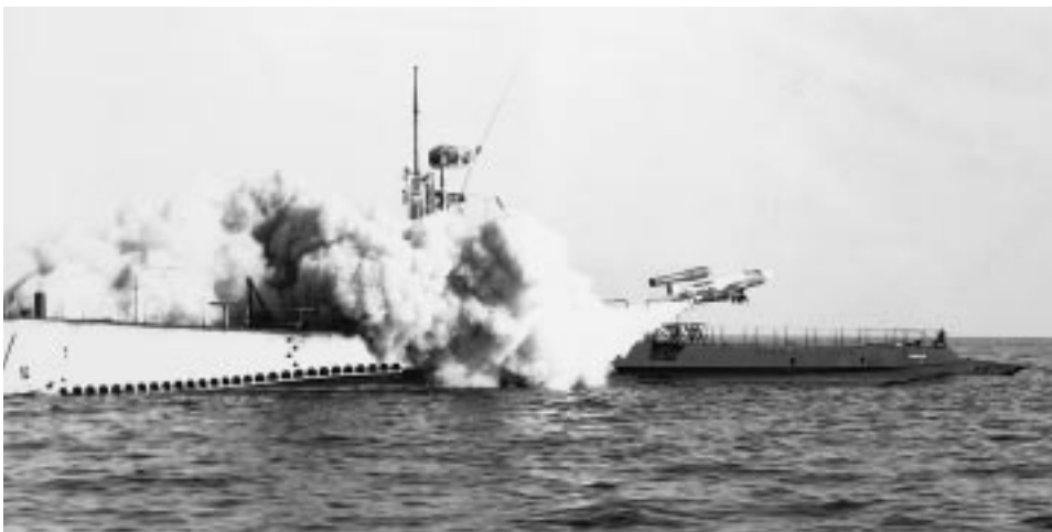
Carbonero launches the Loon, an early step in the adaptation of the guided missile to the submarine 402800
