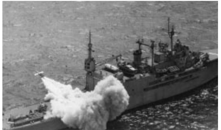
Norton Sound , converted from a seaplane tender to the Navy's first guided missile ship, fires a Loon 415146
