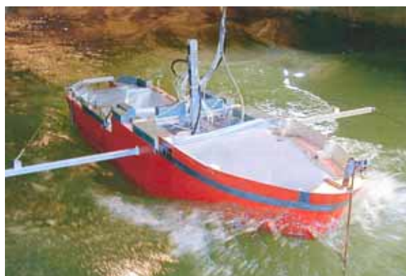
Seakeeping Model Tests of the ARRV. Testing confirmed both excellent sea keeping in the open ocean and the ability to operate effectively in seasonal ice. Credit: Glosten Associates, Inc.
