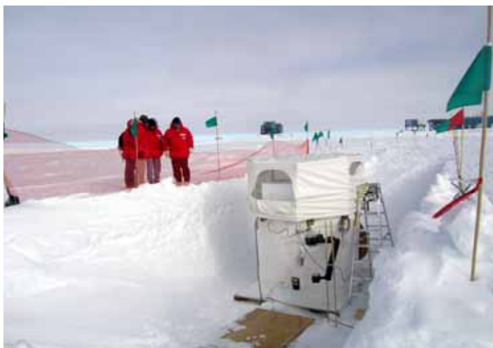
This picture shows the "IceTop" section of IceCube. The deep detector array comprising 4,800 digital optical monitors will be placed at depths up to 2,450 meters in the ice while the surface array, known as IceTop, will comprise 320 DOMs and will be placed at a depth of 1 meter. All components of the array will be connected to a central instrumentation support facility, the Counting House. Credit: the United States Antarctic Program.
