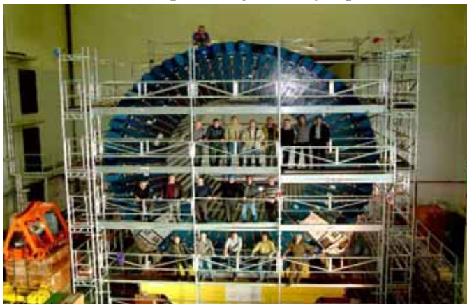
This is a photograph of a partially complete segment of the ATLAS detector. Credit: LHC project.
