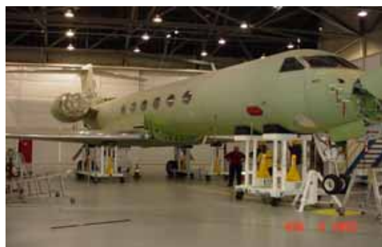
HIAPER - Shored aircraft checked weekly (and often daily) using specialized laser instruments. Credit: National Center for Atmospheric Research (NCAR) and NSF.
