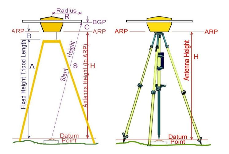
The preferred ARP height determination is made using a tripod with fixed or locking central pole of known height as shown on right above. Other equipment as on left may require computation of the ARP height from slant measurement and/or offsets B or C.
