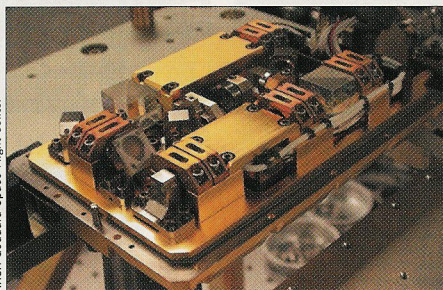
Lightweight laser: the laser weighs 0.56 kg without the beam expander and consumes 8.7 W of power.
