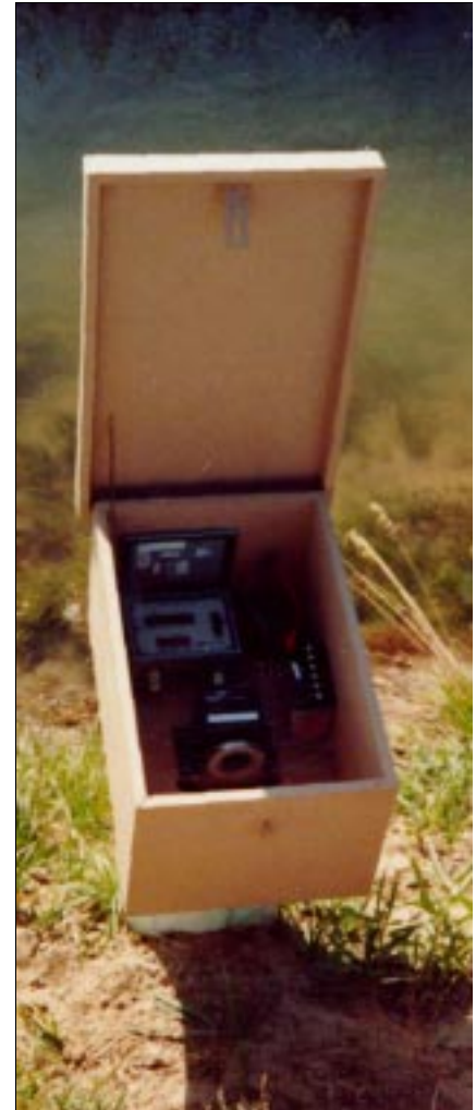
Water measurement devices like this one record the volume of irrigation water delivered.
