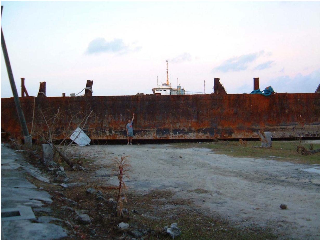
Figure 12. Large ship barge grounded in Colonia Harbor after Typhoon Sudal. The assessment team member in the photo is 6 feet tall.
