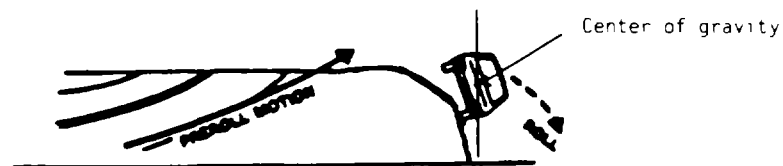
Vertical line through the center of gravity falls outside the vehicle's track
