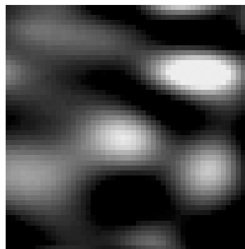
Figure 2. 8 \times 8 \mu\text{m} near-field transmission image of PS/PEA blend film acquired at 2980 \text{ cm}^{-1} . Based on the spectral variation in near-field image contrast, the high transmission features are identified as being PS rich.
