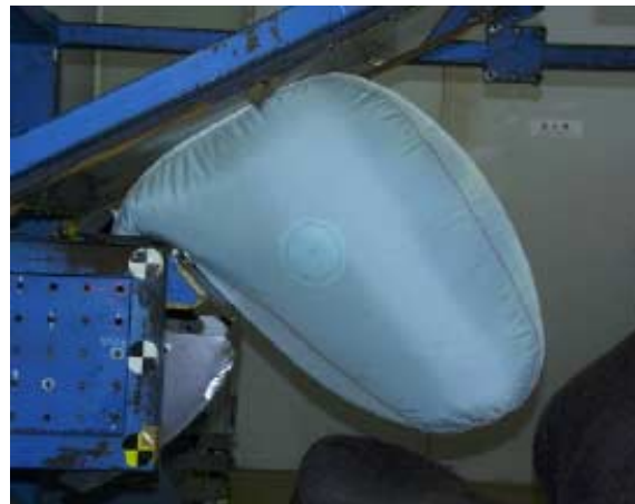
Figure 7. Air Bag Cushion Configuration for Single Stage Module.
