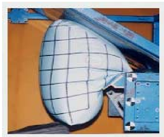
Figure 2. Air Bag Cushion Configuration (Deployed) for Dual Stage Module.
