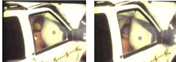
Figures 16 and 17: Illustrations of 5 th percentile female head-to-windshield contact through the passenger air bag and chin-to-instrument panel contact in the Chevrolet Blazer test.
