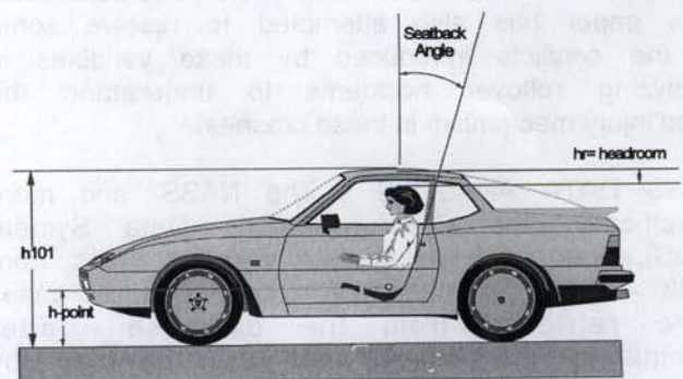
Figure 1. Side view of car with occupant showing headroom.
