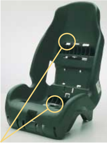
Cosco Booster: After one crash test at 30 mph, there was damage from the restraint harness straps. After a second test, additional deformation of the plastic was observed in places not previously damaged.
