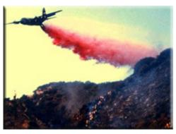
retardant flows to the rear to exit, MAFFS discharges the retardant alternately from a series of tanks to keep the center of gravity within limits. MAFFS-equipped tankers can be re-loaded and flight-ready in less than eight minutes.
