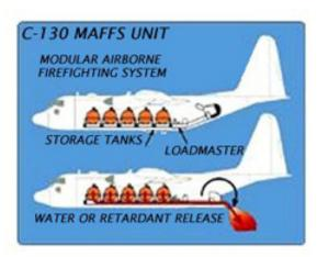
Seven tank modules store the retardant under pressure; each module contains a pressure tank where compressed air is stored at 1200 psi. The control module includes the master control panel, the loadmaster's seat, and discharge valves. An air compressor module
