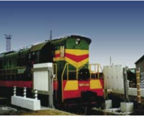
Trains leaving and entering Astrakhan on the Caspian Sea are monitored for nuclear materials as they pass between radiation detectors.
