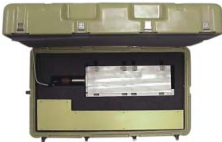
The Adaptable Radiation Area Monitor (ARAM), a portable radiation monitoring system, can detect small amounts of radioactive materials from a distance.
