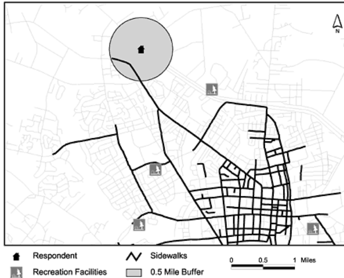
Figure 2. Using a half-mile buffer to represent a neighborhood around a survey respondent's home address, GIS can be used to identify a sidewalk or recreation facility in a survey respondent's neighborhood.
