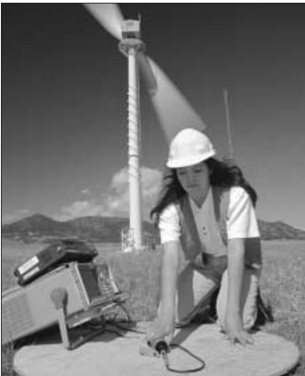
A certification test engineer measures the noise from a wind turbine.
