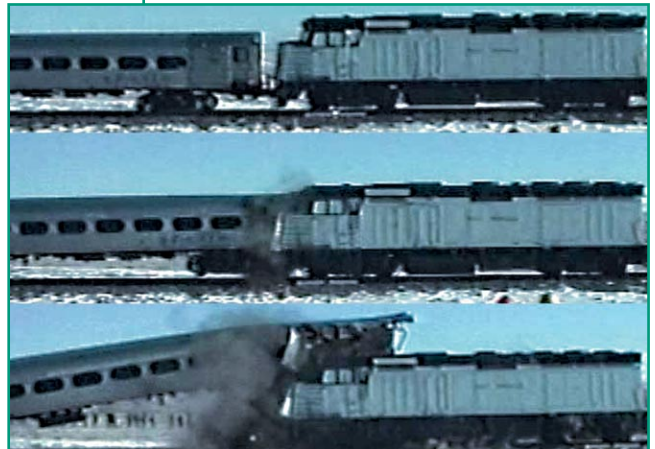
The interaction of the colliding cab car and locomotive recorded during the passenger rail train-to-train impact tests conducted at the FRA Transportation Technology Center in Pueblo, Colorado in January 2002.
