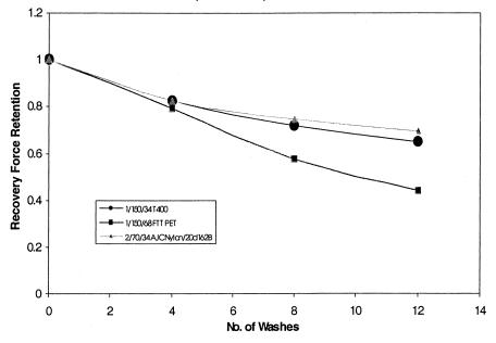
According to DuPont, the data show that the stretch and recovery resulting from the inherent stretch from fiber structure, as represented by the spandex and T400 samples, degrade substantially less than does mechanically induced texturizing in rigid fibers after repeated laundering. When the effect of the lower initial power of the textured fabric is considered, the fabric with T400, after 12 washings, still has approximately 100% of the power of the textured fabric
