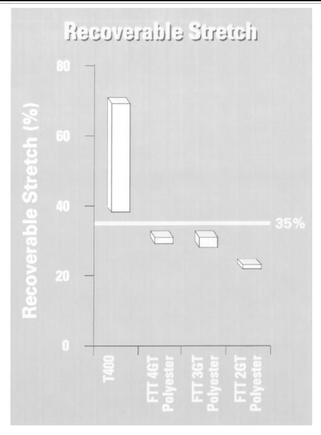
DuPont maintains that the ability of a yarn to recover effectively after being stretched is the key to producing quality stretch fabric. Air jet covered (AJC) spandex yarn (40d spandex with 150d polyester) having 9% by weight spandex was used as a yarn to benchmark recoverable stretch performance to
