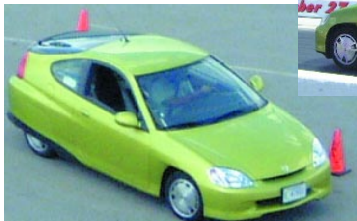
Engineers at Argonne National Laboratory performed fuel economy, braking, acceleration, and handling tests on both the manual and the CVT versions of the Insight.
