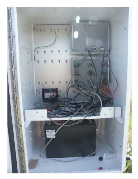
Interior View of RAWS showing FWS-11 Data Logger. All of the data from the sensors is stored here.
