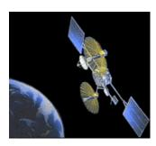
Currently 24 GPS Satellites in orbit. Provide continuous 3-dimensional position, velocity, and time information for users with GPS receivers anywhere on or near the earths surface. Our RAWS stations utilize the Lat/Long Coordinates and GPS clock timing.
