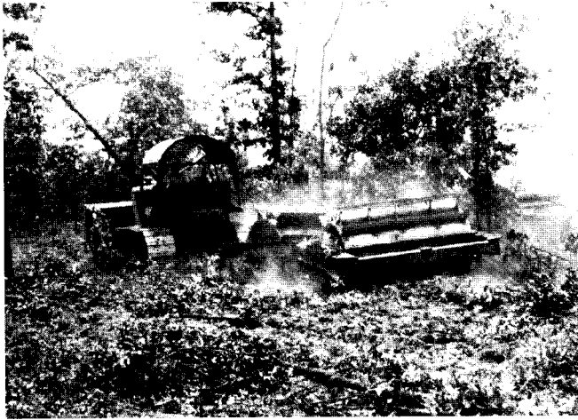
Figure 4-3 —Chopping an upland scrub hardwood site with dual, offset, 1 O-t choppers pulled by a D-8 tractor.
