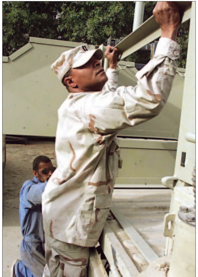
[Right] Capt. Darryl M. Butler, a facility engineer with the 354th Civil Affairs Brigade, Riverdale, Md., inspects a new Modified Protection for un-Armored Humvees kit (MPAH) before it is lowered onto a Humvee. Butler, the kit's designer, personally oversees the installation of each kit.
