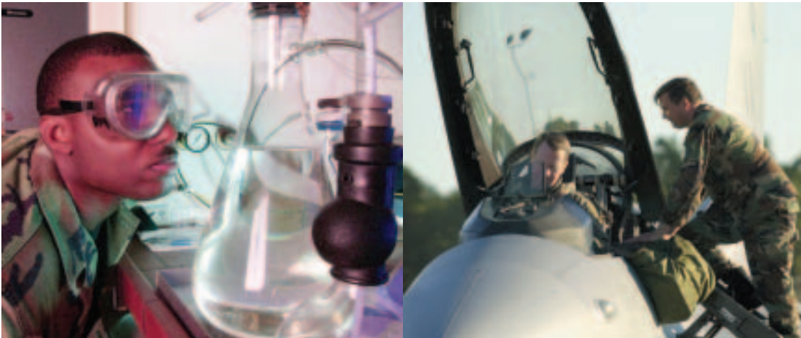
SrA Rickett Edwards, a fuels specialist from the 374th Supply Squadron/Fuels Management Flight, Yokota Air Base, Japan, performs an icing inhibitor test on JP-8 fuel. The laboratory conducts more than 500 tests monthly.
