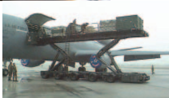
The Tunner 60-K loader dramatically expedites the handling and processing of cargo pallets for our strategic airlift fleet. Tankers such as the KC-10 (above) and the KC-135 (left) are critical enablers for that strategic airlift.
