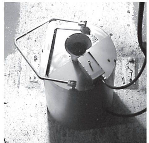
The Research Reactor Spent Fuel Counter underwater in the Savannah River L Basin.
