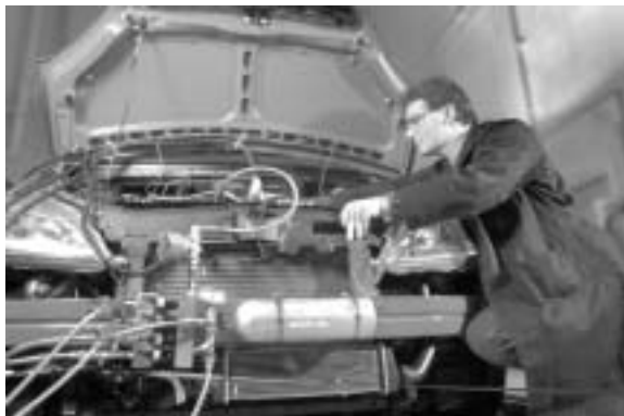
Scott Sluder, ORNL, checks the components of an experimental diesel emission control system before checking its effectiveness on a vehicle dynamometer. Diesel engines are inherently more fuel-efficient than gasoline engines, but present challenging emissions issues.
