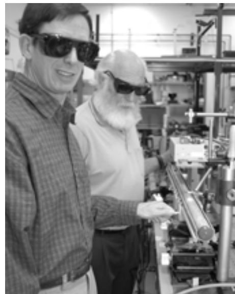
David Cremers (left) and Monty Ferris of Advanced Chemical Diagnostics at Los Alamos National Laboratory, use Laser-Induced Breakdown Spectroscopy to determine the amount of carbon in a sample of soil contained in the tube.
