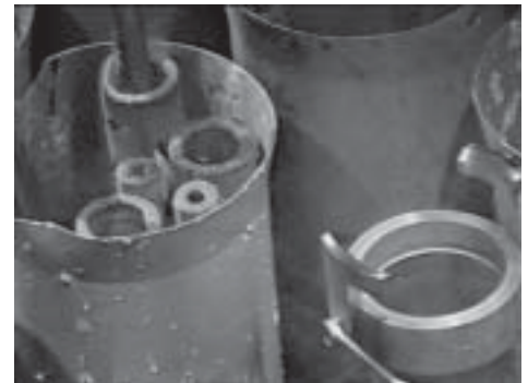
Spent nuclear fuel stored under water at the Hanford Site.
