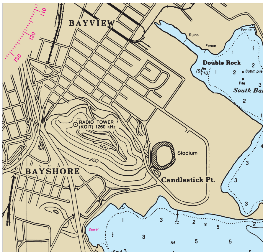
Fig. 3-4. Excerpt from NOS Chart No. 18650 (San Francisco Bay), showing contour lines on hill near Candlestick Park
