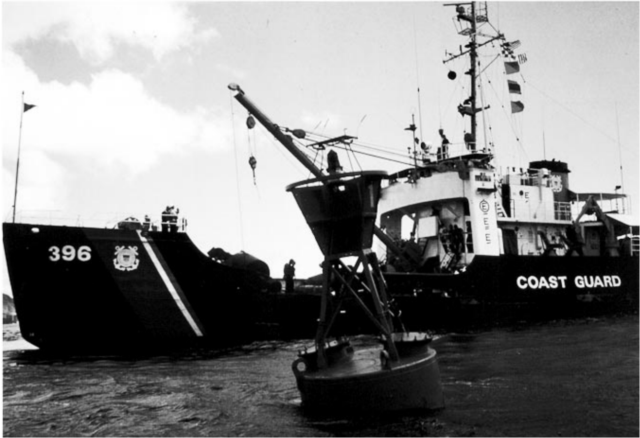
U.S. Coast Guard Buoy Tender passing by green-lighted radar-reflective buoy. Angle of buoy suggests current is moving from right to left in this photograph. Approximately 4,600 lighted buoys mark U.S. waters. Official U.S. Coast Guard photograph.
