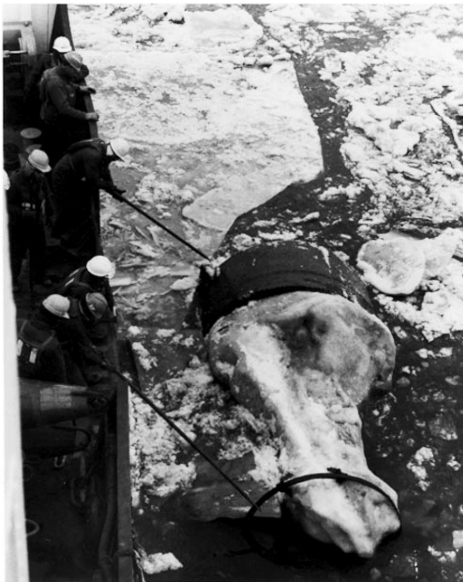
Buoys can be damaged and moved off station by ice, one of the reasons that position-fixing with buoys is not recommended. Here crew from the USCG Red Oak work on an ice-damaged buoy. Official U.S. Coast Guard photograph.
