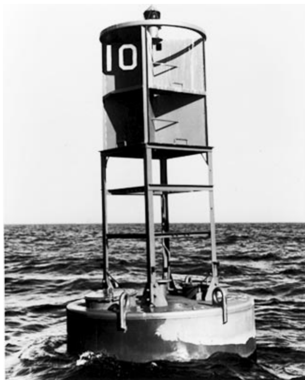
A Standard Lighted Radar Reflective Buoy (no sound). Official U.S. Coast Guard Photograph.
