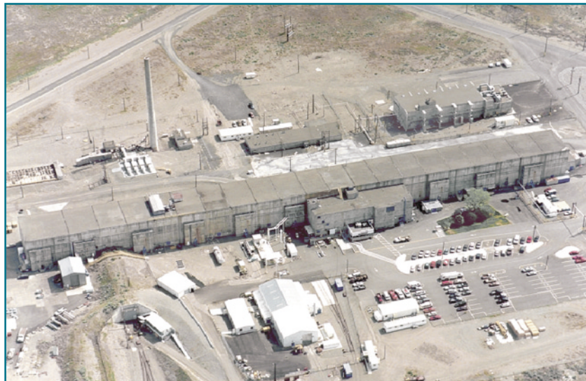
Figure 4. The T-Plant chemical separation facility used the bismuth-phosphate process to recover plutonium.
