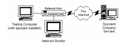
As shown in the diagram, all communications from the computer with spyware installed must pass through a network hub on their way to the Internet. My network monitor computer, also connected to that hub, sees all such communications and preserves them for my subsequent review.
