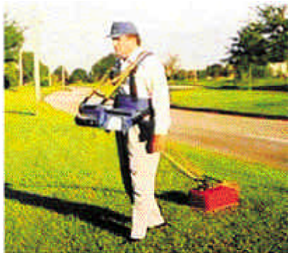
Figure 8. Using GPR on a ground survey
