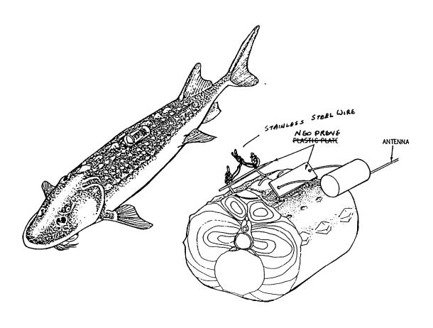
$Figure \ 5. \quad Attachment \ of \ external \ radio \ transmitter \ to \ white \ sturgeon.$
