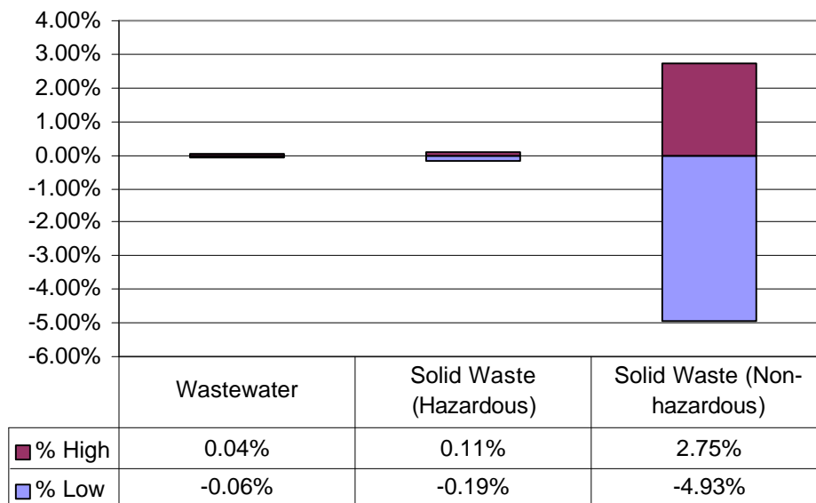
Figure 22: The Effect of Soybean Oil Conversion Energy Demands on Water and Solid Waste Emissions for Biodiesel
