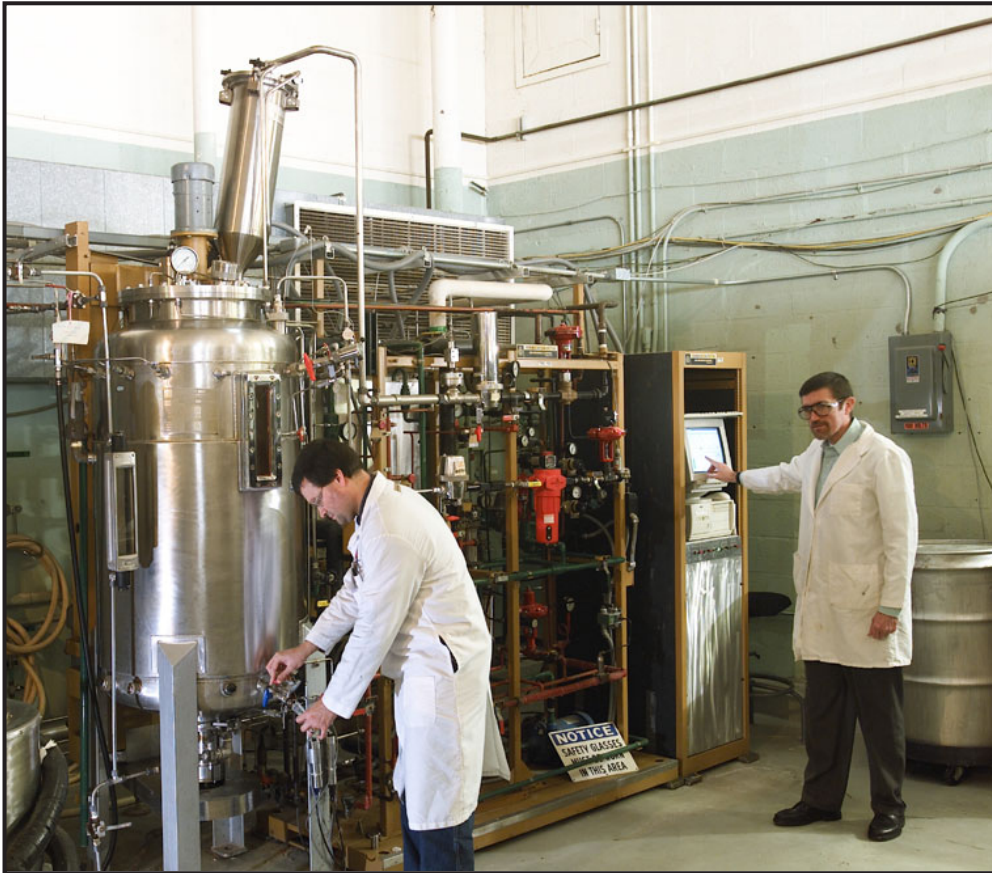
A 500-L computer-controlled fermentor for large-scale production of microorganisms.
