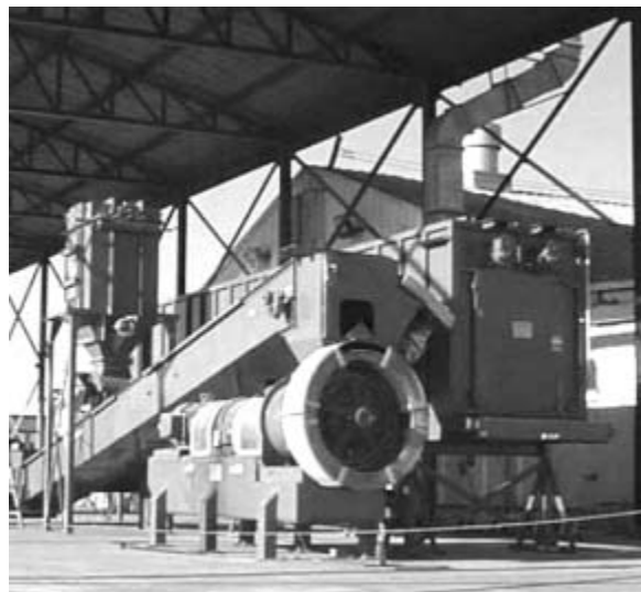
Figure 9. The PEF Facility has a shredder and a cubing machine to convert waste paper into cubes used for fuel in SRS stoker boilers.
