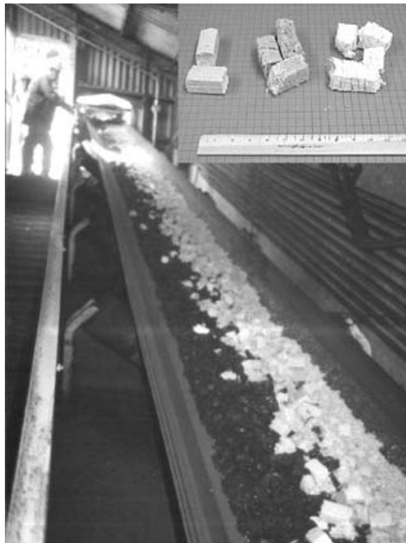
Figure 10. The combined feedstock material is processed through a machine that extrudes it into cubes approximately 1 in. square and 3 to 4 in. long. Sample cubes shown in the inset (left to right) are made of wood, cardboard, and office paper.
