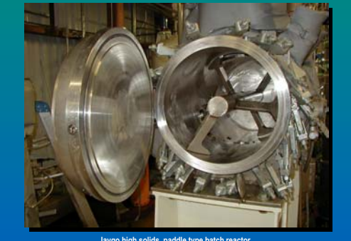
Jaygo high solids, paddle type batch reactor.
