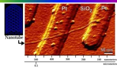
Nanotubes exhibit unique quantum-wire properties which derive from their nanometer diameter and the special electronic structure of graphite. Nanotube transistors have recently been fabricated. These three-terminal devices consist of an individual semiconducting nanotube on two metal nanoelectrodes with the substrate as a gate electrode.
