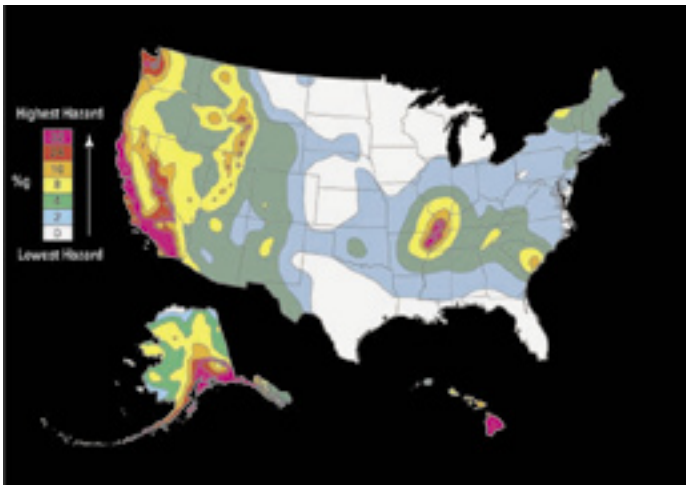
U. S. Geological Survey Earthquake Hazard Map for the United States showing areas in the country where earthquake hazards are the most (in red and orange) and least (white). This map is based on known seismic activity and the long-term rates that faults are moving. It takes into account how often earthquakes occur in a given area and at what magnitude. Some local areas may face higher hazards due to they way local geology and soils may make earthquake shaking worse
