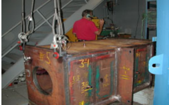
HSLA-100 Steel/LC-100 Weld Metal Box-Tank Fatigue Model Overall View of Model Exterior/End Hatch Open
