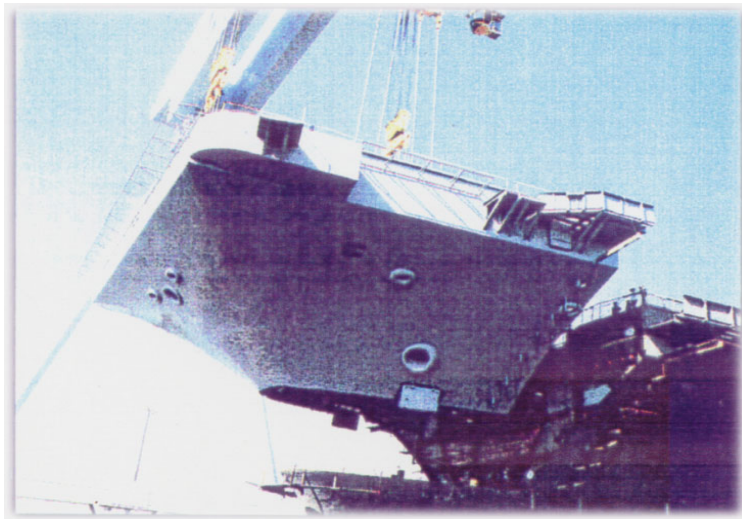
CVN 74 HSLA-100 Steel Main Deck Panel Fabrication
