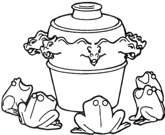
Chinese seismoscope, 132 A.D. The direction in which the first ball fell was thought to indicate the direction of the epicenter.
