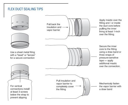
Connections between the air handler cabinet and the main supply and return plenums or ducts should be sealed with mastic or approved pressure-sensitive tapes. It is sometimes easier to remove service panels and seal these areas from the inside using mastic.
