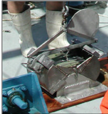
Figure 6. The modified ponar grab used for sediment collection.
