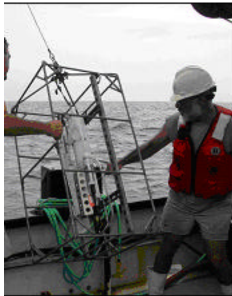
Figure 5. Deployment of the Seabird for water quality assessment.
