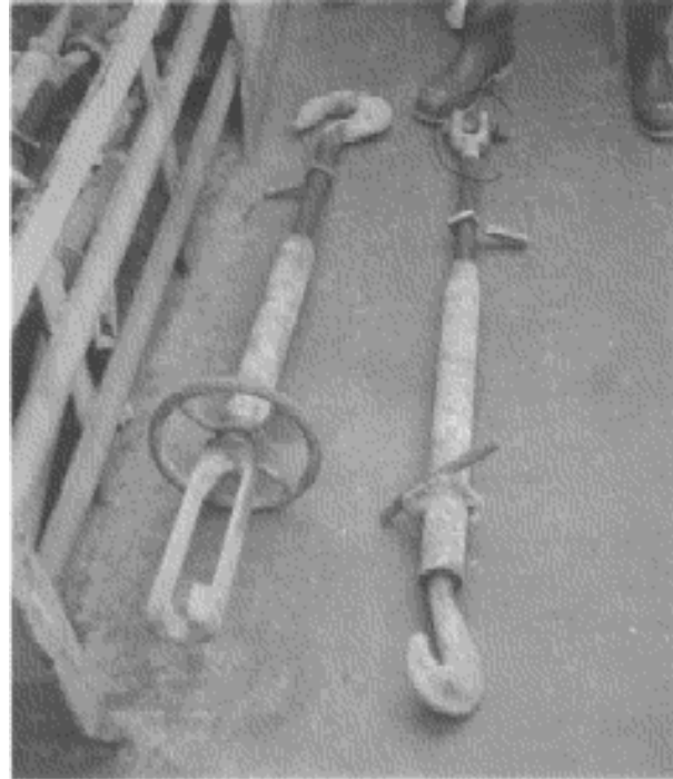
Two types of turnbuckles onboard SANTA CLARA I (cylindrical claw on left; rigid hook on right)
