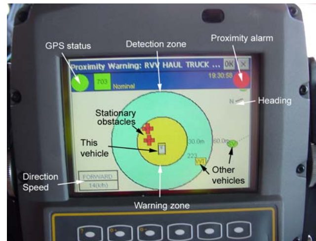
Figure 7. Driver interface for GPS-based proximity warning system.
