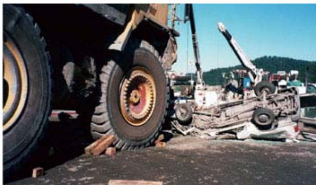
Figure 1. Accident involving collision between off-highway dump truck and van.
