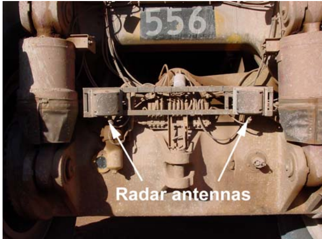
Figure 3. Preview radar system with two antennas.
