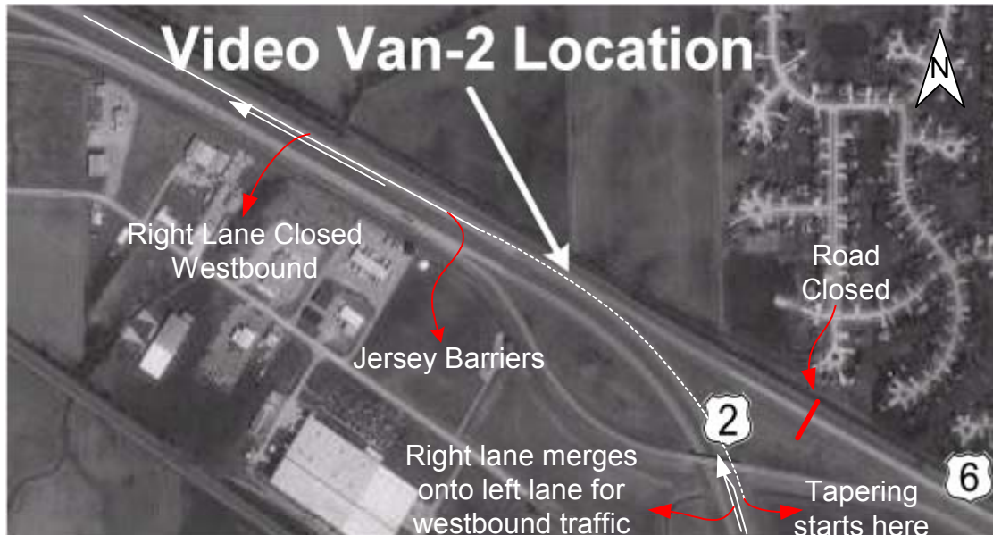
b. Cambridge Workzone, Aerial view of the approximate location of the I-70 eastbound lane closure, before construction.
