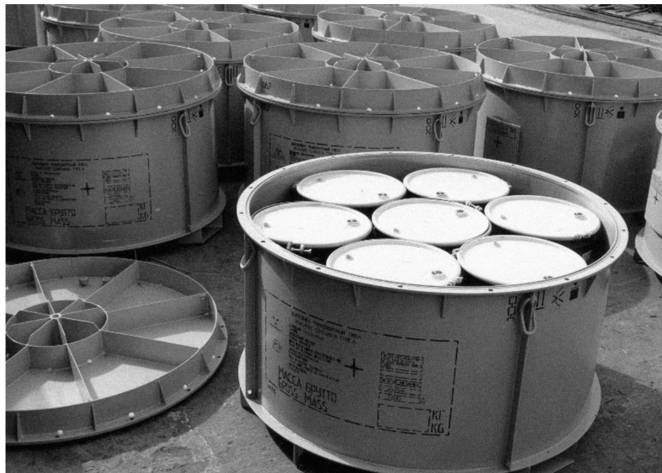
Figure 5: Steel Containers Used to Store Solid Radioactive Waste from Dismantled Submarines
