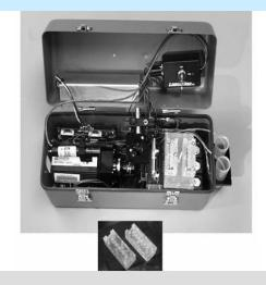
Figure 14 – The most recent version of the NRL array biosensor with integrated optics and fluidics components. Six-reservoir modules for holding samples and fluorescent tracer reagents are shown separately below. Source: Dr. Frances S. Ligler and Chris R. Taitt, "The Array Biosensors." Received June 1, 2004.
